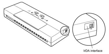
**2.** Locate the IrDA interface on the computer. Arrange the printer so the IrDA interface ports are facing one another.
